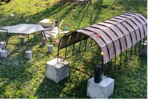
Figure 2: Image to show Spider pod and Arch pod frames used for 'control site' at Koh Bong for Artifical reef and recruitment studies.
